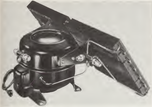
16-12. A natural convection finned condenser. This unit has two service valves. The condenser is inclined to permit cool air to contact all parts of the condenser. (Tecumseh Products Co.)
